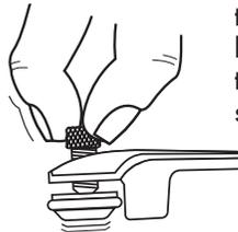
You can fine-tune how tightly the Hoop Clamp holds the hoop by adjusting the hoop tongue adjuster screw, as shown on the left.
