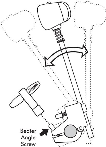
The Beater of the Dyno-Matic Pedal can be positioned independently - without affecting the positions of the Pedalboard, the Spring Arm, or the Axle height. The forward, or backward angle of the Beater Cam is adjusted by loosening the Beater Angle Screw with the Drum Key, as shown on the left. The length of the Beater shaft can be changed by loosening the Beater Length Screw with the Drum Key, as shown on the right. Be sure to tighten the screws securely once positioned.
